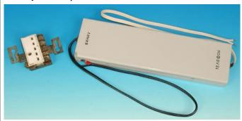
TF-B tx (5) Pschola transmitter (bug) 33020-11 fitted in a Variant terminal box (left) and Peperuda receiver (right).
